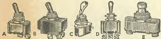
Fig. A—SINGLE POLE SWITCHES
